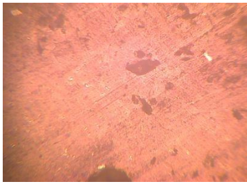
.Fig 2: Microstructure of 2wt% mica 2wt% e-glass fiber, Al6061 Composite specimen
